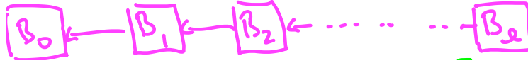
Figure 10: When there are no message delays or Byzantine nodes, there are no forks.
